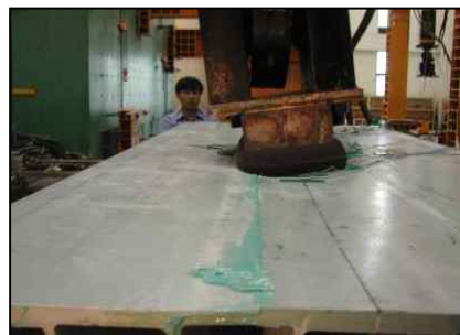
Failure at 412kN [F.S.=3.4 for DB24 Axle Load(122kN, 1.33xASHTO_H20)].
