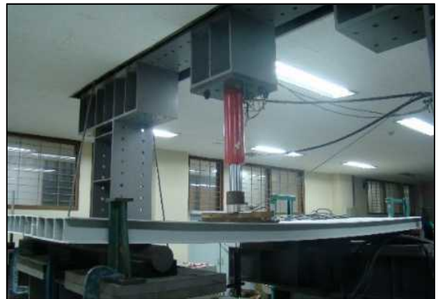
Flexural Test of SF75L Deck (2m-span S.S Beam). Failure at 6 Times of Footbridge Live Load, 5KN/m 2 (F.S.=6). Deflection: 1/2 of Serviceability Limit.
