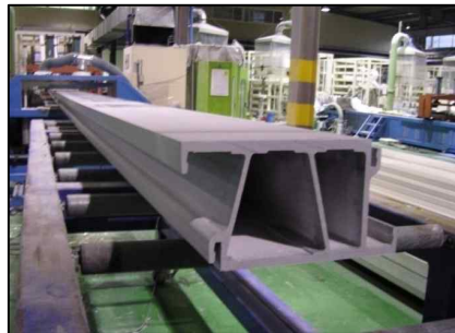
Pultrusion of SF200 Deck
